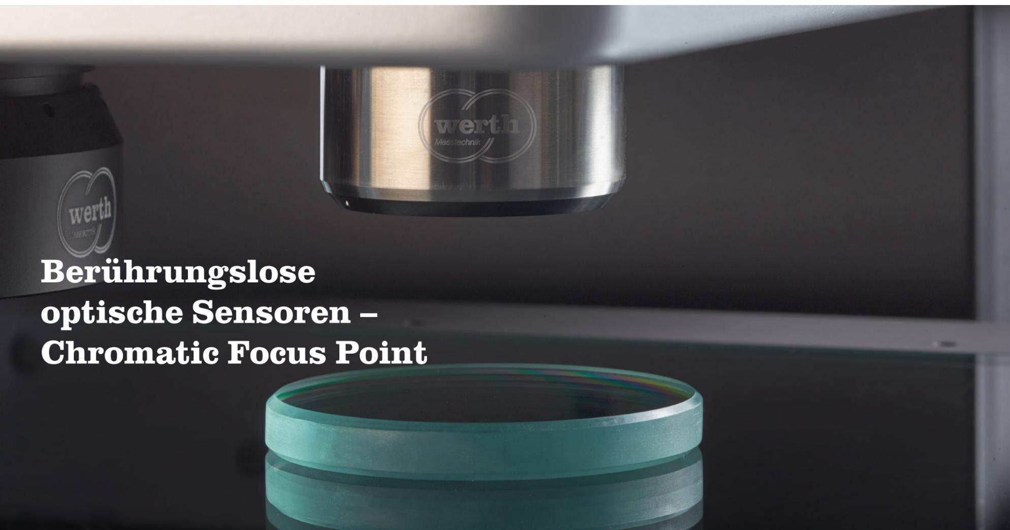
A close-up photograph of a Werth Chromatic Focus Point sensor. The sensor is a cylindrical metal component with a polished, reflective surface. It is positioned above a green, ring-shaped workpiece. The Werth logo is visible on the side of the sensor. The background is dark and out of focus.
