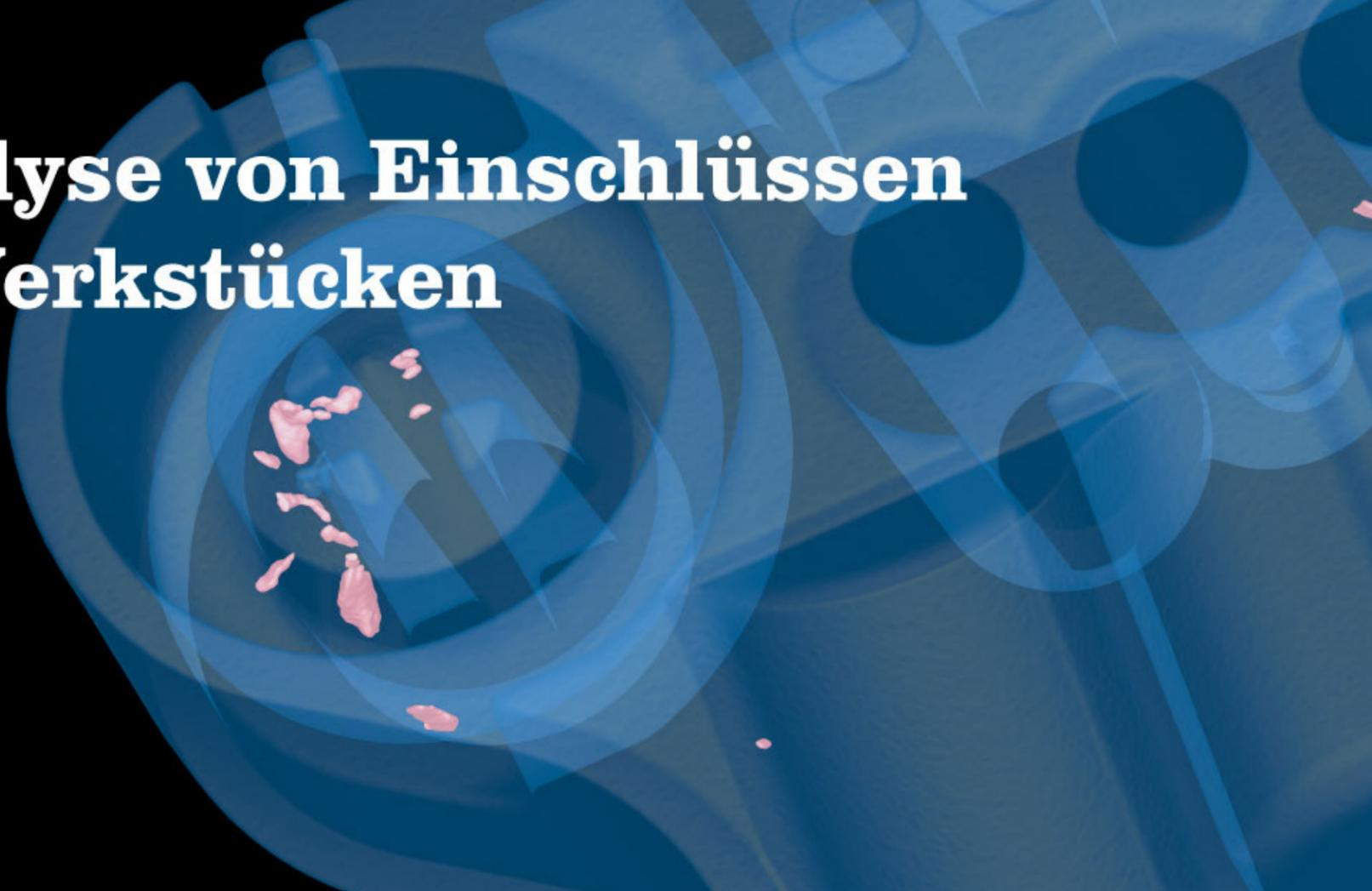
A 3D visualization of a mechanical part, likely a gear or a similar component, rendered in a semi-transparent blue. The interior of the part is visible, showing several irregular, reddish-pink shapes that represent internal defects or inclusions. The background is dark, making the blue part stand out.
